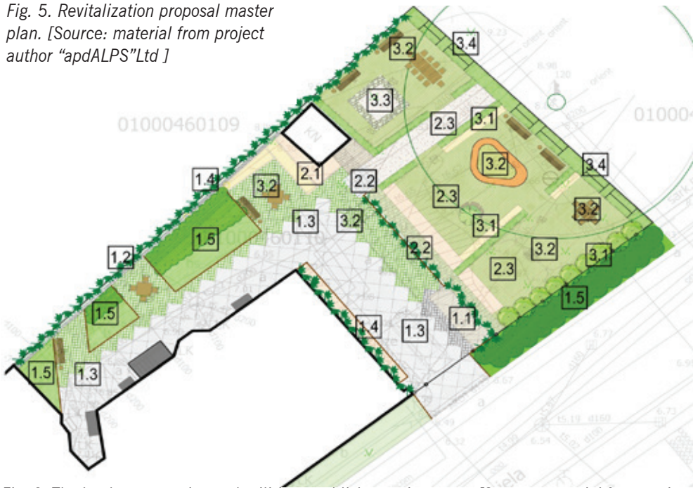
Fig. 6. The landscape service and utilities establishment in stages. [Source: material from project author "apdALPS" Ltd.], with the following designations: Stage 1 — 1.1. Construction of housing for waste containers; 1.2. Construction of support walls; 1.3. Construction of access road surface; 1.4. Planting climbing plants along the support walls and walls of the building; 1.5. Lawn installation, incorporating ground cover plants; Stage 2 — 2.1. Creating high beds and plantings; 2.2. Installation of gabion retaining walls and stair construction; 2.3. Terrain levelling, pavement construction, and lawn installation; Stage 3 — 3.1. Plantation of greenery in courtyard "rooms"; 3.2. Installation of playground equipment, garden furniture and bike shelter; 3.3. Construction of campfire pits; 3.4. Hedge planting along the fence.
